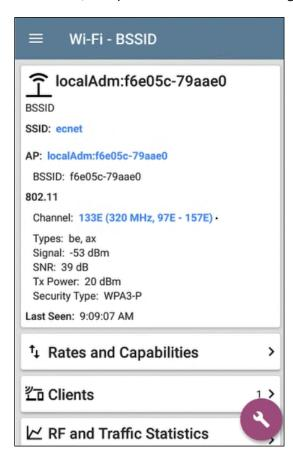
If your tester detects Wi-Fi 7 traffic, related Sort and Filter options for **320 MHz** channels and 802.11**be** are displayed.
